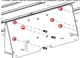
1. Assemble as shown using **6 x M6x12** screws, then attach this assembly to top of F50 floor stand.
