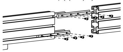
1. Fix wall mount as shown using 6 x M6x12 screws
