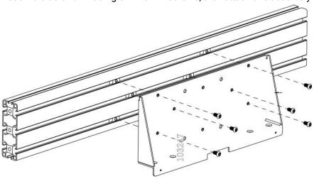
2. Join rails. Note for smaller displays you may only need two of the three sections.
