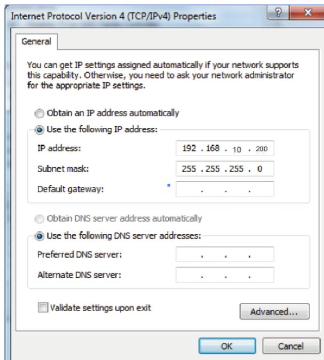
**Notice:** The IP address of the computer and Transmitter should be in the same network segment. As the Transmitter’s IP address is 192.168.10.10, the computer’s IP should be 192.168.10.X (X contains 1~255 except 10).
