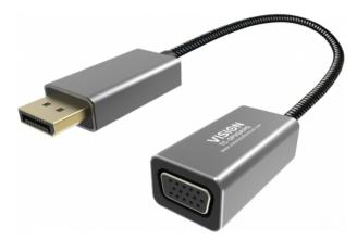
Plugs into DisplayPort on laptop and has VGA socket. Active circuit converts the digital signal into analogue VGA for display devices which don't have a digital input.
