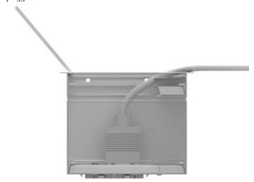
If you'd prefer to mount the surround in the top position remove the long side opposite the hinge and reassemble:
