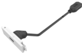
TC3 HDMI [SAP:3446573] HDMI module 1.4 AWG 28 - tail 200mm (7.87") long
