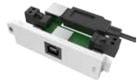
TC3 USBB+ [SAP:3446582] USB-b module with active booster circuit. USB 2.0 Maximum input cable length: 10m. Note: Uses 5v from USB. For longer cables external power may be required.
